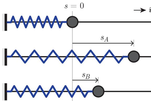
Figure 2.9: Spring acting on an object as it moves along a straight line.
