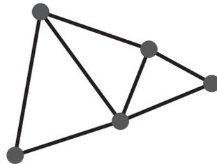
Figure 4.2: Rigid body consisting of discrete particles connected by massless rigid rods.
