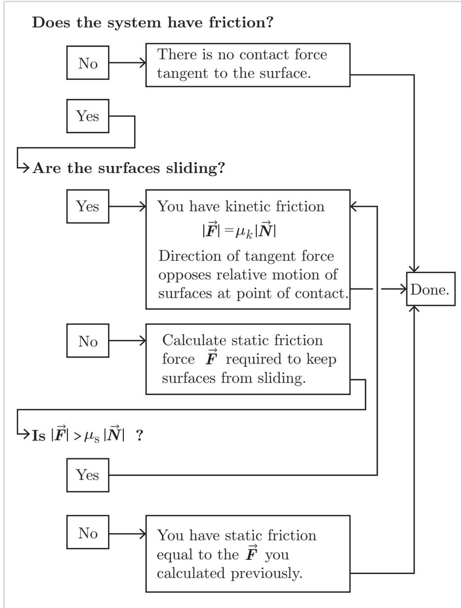
Figure 2.4: Implementation of the Coulomb friction model.
