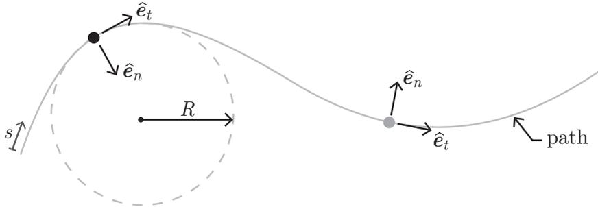
Figure 1.2: Motion along a curved path.
