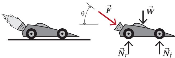
Figure 2.7: Rocket car with constant thrust force  $\vec{F}$ .
