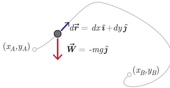
Figure 2.8: A path over which to calculate work by gravity.
