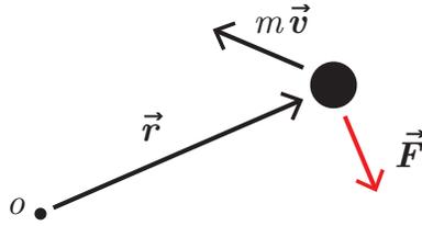
Figure 3.1: Elements of the angular momentum.
