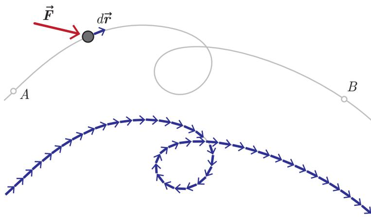
Figure 2.6: Work is a path integral.
