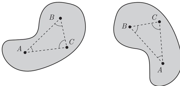
Figure 4.3: Rigid body with a continuous distribution of mass.
