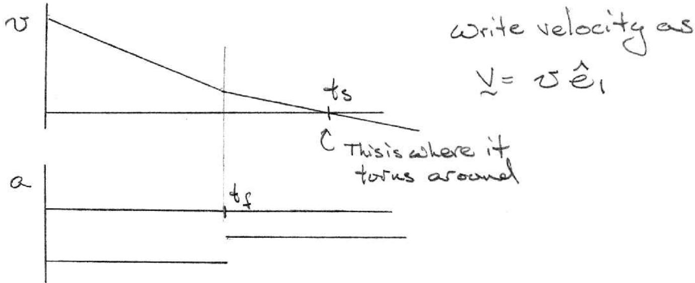
Kinematics while on friction part  $0 \leq t \leq t_f$
